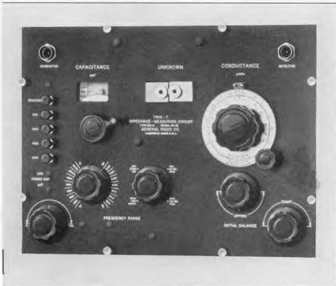
FIGURE 4. Panel view of experimental model of Twin-T impedance-measuring circuit. At the left of the panel are the susceptance condenser (CAPACITANCE \mu\mu\text{f} ) and the auxiliary tuning condenser (AUX. TUNING CAP.). At the right are the conductance condenser (CONDUCTANCE \mu\text{mho} ), and the parallel trimmer condensers (INITIAL BALANCE). The remaining controls (FREQ. RANGE) are the coil switch, at the left, and the conductance range switch, at the right.
