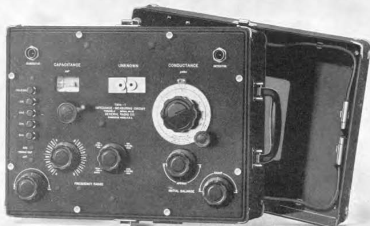
FIGURE 1. View of the TYPE 821-A Twin-T Impedance-Measuring Circuit with cover removed. The airplane-luggage type of case is provided with a carrying handle and the instrument is easily portable. Connecting cables and instruction book are mounted in the cover.
