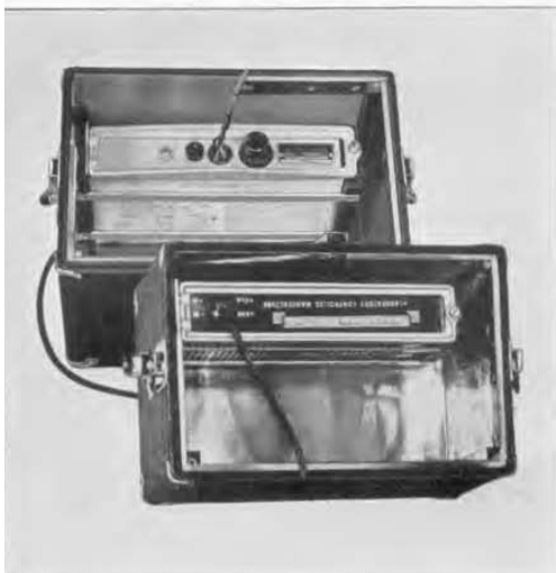
FIGURE 8. Both the TYPE 759-P50 Power Supply Unit and the Burgess type 6TA60 battery may be used interchangeably in the TYPE 759-B Sound-Level Meter, as shown here.
