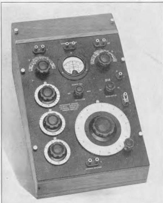
FIGURE 1. View of the TYPE 650-A Impedance Bridge with battery compartment at the rear.
