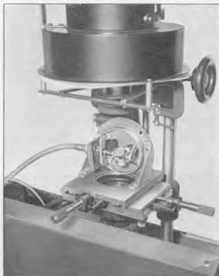
FIGURE 1. View of the tachometer mounted in the contour comparator with Strobolux lamp above.
