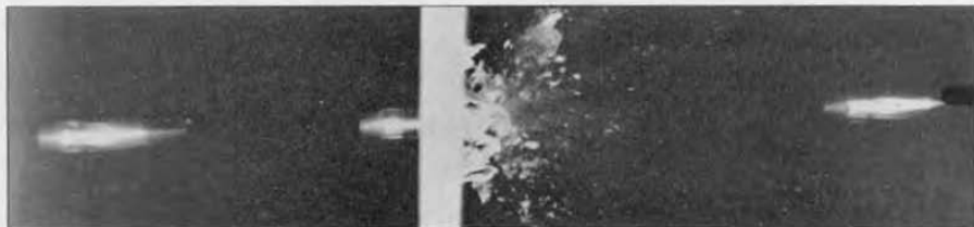
FIGURE 1. Three-exposure photograph of a 0.50 caliber machine-gun bullet.
