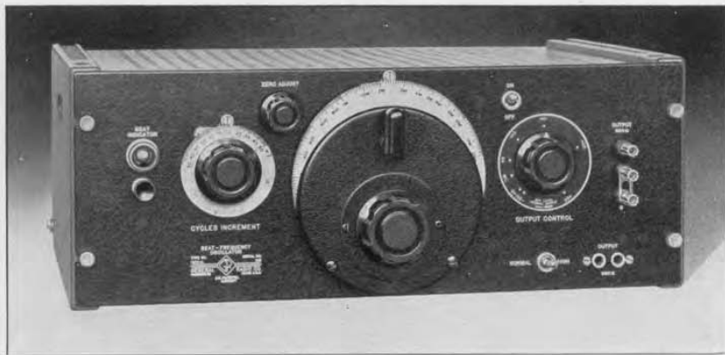
Figure 1. Panel view of the Type 1304-A Beat-Frequency Oscillator. New features include an illuminated, precision-type, main dial, and an incremental frequency dial with a range of -50 to +50 cycles.
